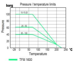
Note: Working pressure may be limited by the valve connections.
