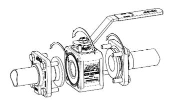
Loose body flanges make it possible to install the valve without the aligning of welded end connections. After installation the valve can rotate 360° for the desired orientation.
