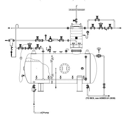
In systems where condensate return is negligible and/or high flow rates are involved, an additional dome steam injection should be provided.
