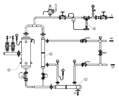
The condensate return (CR) is expanded on a flash vessel (3). The flash steam which is produced there and the remaining condensate are then directed to the respective heat exchangers (1 e 2) where, in the meanwhile, the pressurized feed water (CW) is heated (HW) before it passes to the economizer or is directly introduced in the steam boiler (it is recommended to install a by-pass from CW to HW).
