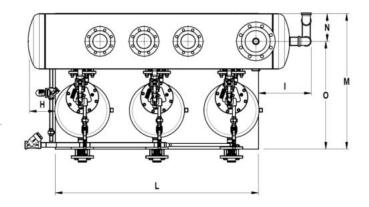
LIMITING CONDITIONS: Receiver - Max. operating pressure: 0,5 bar. Pump: See IS 9.101 E.
