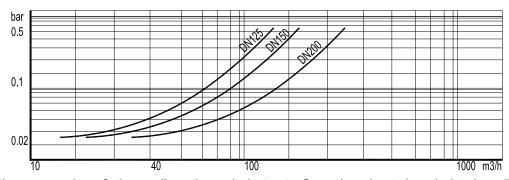
To determine the pressure drop of other mediums the equivalent water flow volume has to be calculated:
