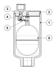
PMO – Max. operating press.: 30 bar; TMO – Max. operating temp.: 300 °C;
